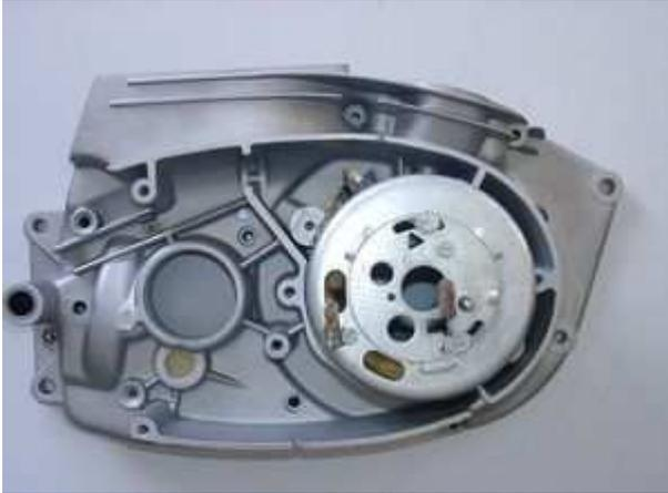
Disconnect all cables from your old generator, regulator and the ignition coils and remove those parts. You may pull your old rotor from the crankshaft by means of a puller screw M8x90.
