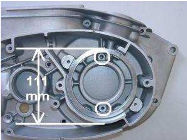
Place the outer adapter ring into the crank casing, where your old magneto had been sitting.
