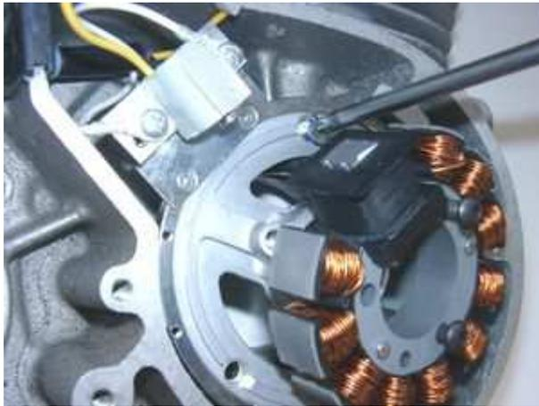
Put the base plate (consisting of the outer steel ring and the inner aluminium plate) into the place of your old generator.
