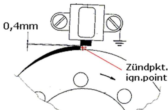
Turn the rotor slowly by hand and check clearance between the sensor and one of the rotor noses. This has to be ca. 0,4mm. You may adjust the gap by loosening the 2 holder screws of the sensor and shifting it a little. Do not forget to tighten the 2 holder screws of the sensor carefully. If loose, the sensor will get into contact with the rotor and will be destroyed. It is a good idea to check secure fitment from time to time.
