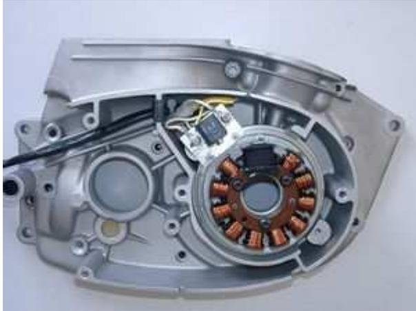
This is how the installed stator unit will look like.
