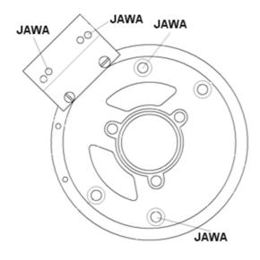
Unscrew the stator coil from the base plate and lift it a little away from it so that you can access the mounting holes. Take care not to damage the paint insulation of the coil. Identify the correct fastening holes at the baseplate as seen here. There are 2 sets of them, one used for all JAWA models.
