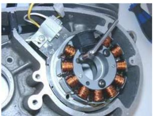
Put the stator coil back onto the plate, take care not the damage the wires.
