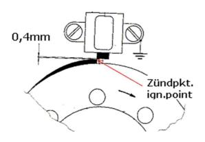
Turn the rotor slowly by hand and check clearance between the sensor and one of the rotor noses. This has to be ca. 0,4mm. You may adjust the gap by loosening the 2 holder screws of the sensor and shifting it a little. Do not forget to tighten the 2 holder screws of the sensor carefully. If loose, the sensor will get into contact with the rotor and will be destroyed. It is a good idea to check secure fitment from time to time.
