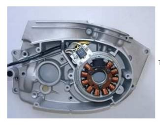
This is how the installed stator unit will look like.
