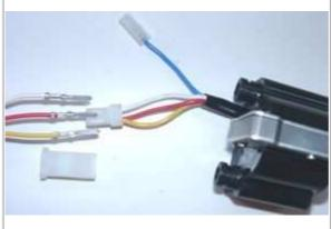
Look for the ignition coil with its female plug and the three wires (red, yellow and white).
