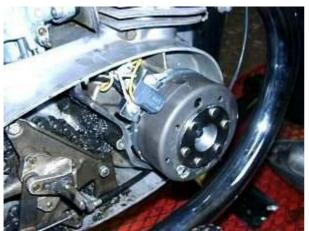
Place the rotor drum onto the crankshaft, taking care to fit the slot onto the roller pin of the crank. Check that the rotor sits well on the shaft. It happens that a roller pin is a little to high and prevents good fitment. In that case take a little material of the roller.
