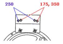
For the **250cc** the sensor will be positioned to the LH side.
