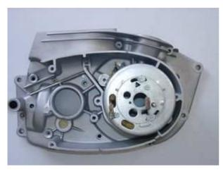
Disconnect all cables from your old generator, regulator and the ignition coils and remove those parts. You may pull your old rotor from the crankshaft by means of a puller screw M8x90.
