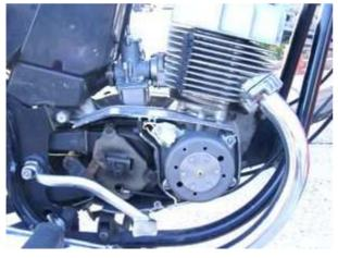
Place the new rotor onto the crankpin. Make sure that the arresting pin sits in the rotor's groove and the rotor sits tighty on the shaft. To pull the rotor again (when needed) use a simple screw M12 as a puller.
