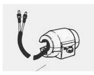
Disconnect the engine stop switch at the righthandside of the handlebar from plus and reconnect it to ground.
