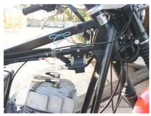
Fasten the new ignition coil with its holder at the frame under the tank. Try to put this coil as far as possible to the front (and away from the heat of the cylinders).
